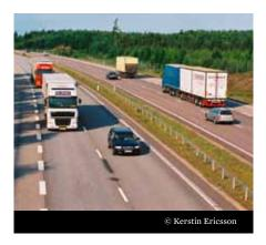
• **Speed limits** on parts of the road network have been reviewed in order to ensure that they reflect the safety standard of the road. For example, there are now few roads with a speed limit of 110 km/h that do not have a median barrier.
